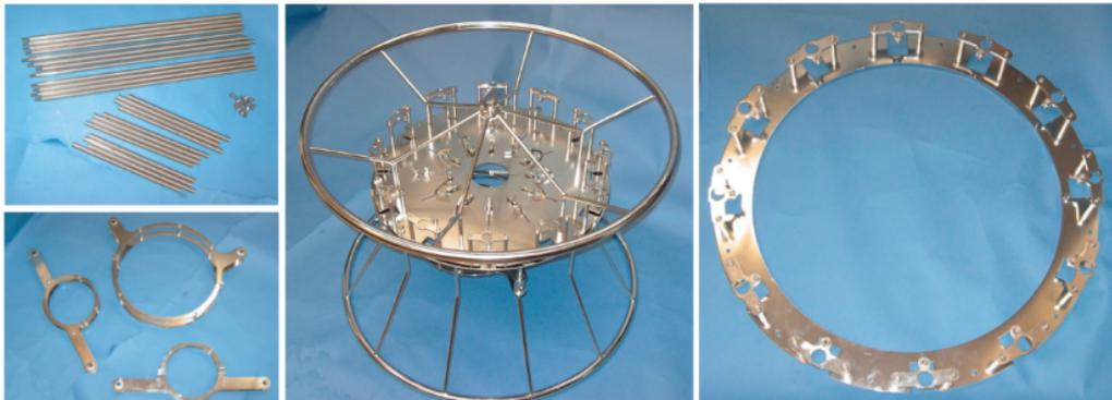
Begin by separating the top and bottom frames, by undoing the wing nuts holding them together:
