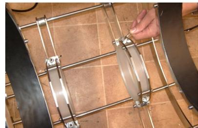
Each clamping bracket is made of two half-clamps. These should be separated by undoing the screws as shown: The MIDAS CTD+ is shipped in a separate frame, which may be used for deploying the instrument on its own if required.
