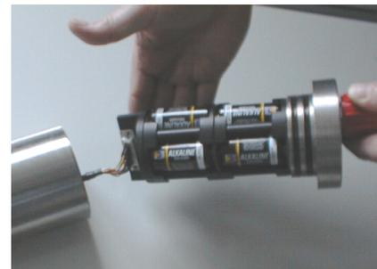
5. A lead connects the battery pack to the electronics inside the tube. This may be disconnected at the battery pack if required, for ease.
