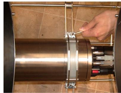
Repeat this procedure to fit the EcoLab system into the large clamps.
