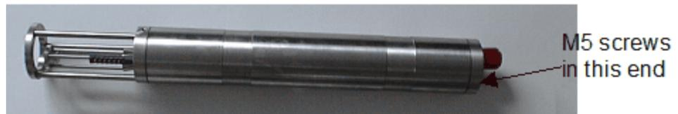
3. Remove the 3 M5 x 20 socket cap screws in the connector bulkhead, using the Allen key provided. Note that these screws are titanium, and should be replaced with titanium screws if lost. Other materials may suffer galvanic corrosion and may be destroyed.
