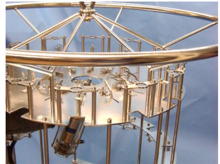
If the rotor arm is loose, it must be secured in the correct position. To do this it is necessary to communicate with the instrument using the software. This procedure is therefore described in the software manual.
