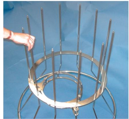
Lower the instrument clamping brackets onto the rods. The larger EcoLab bracket should be positioned vertically above the bracket that is already in place. The smaller MIDAS CTD+ brackets should be positioned directly opposite the EcoLab brackets, vertically above each other.
