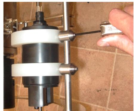
Next, place the bottle mounting ring on the rods, taking care to position it the right way up. The thread on the top of the rods should fit through the holes in the ring. Then, screw the 20cm rods in place as shown, tightening as much as possible.
