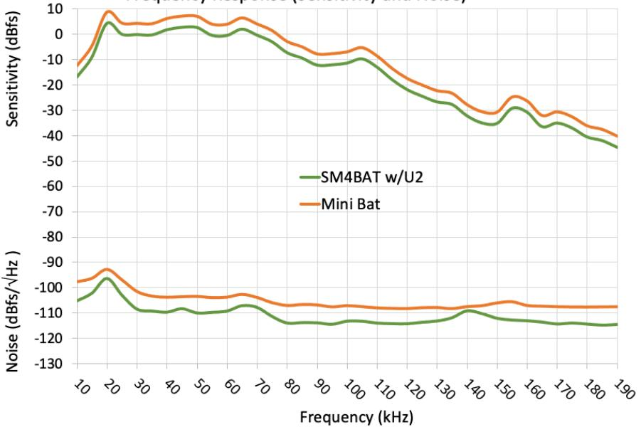
SM4BAT w/ SMM-U2 and Mini Bat On-axis Signal To Noise Ratio
